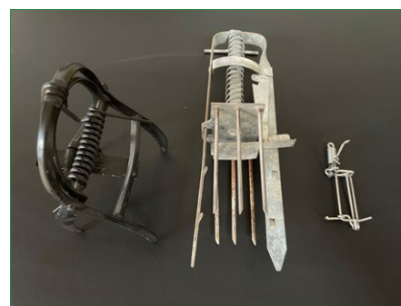
Figure 4. Common mole trap designs include scissor-jaw, harpoon, and pincer (from left to right).
